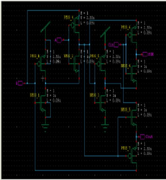
Fig. 6: Full Adder construction in Tanner EDA tool
