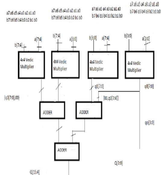
Fig. 2: 4-Bit Vedic Multiplier Architecture
