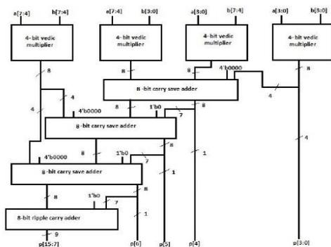
Fig. 4: 8-bit Vedic Multiplier Architecture
