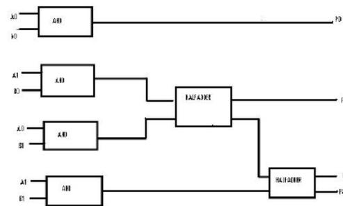
Fig. 3: 2-bit Vedic Multiplier Architecture
