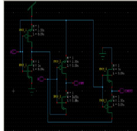
Fig. 5: Half Adder construction in Tanner EDA tool
