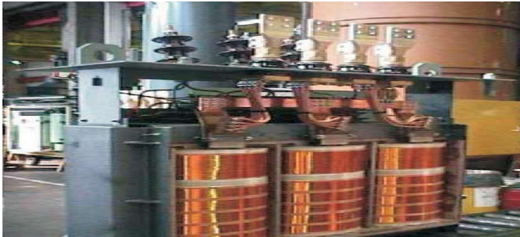
Fig8: 1600 kVA Amorphous Core Transformer
