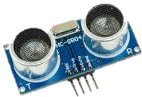
**Figure 5: HC-SR04 ULTRASONIC SENSOR**
