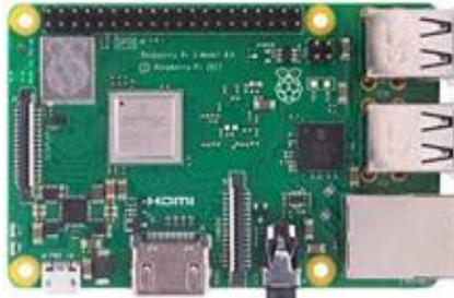
*Figure 2:Raspberry Pi 3 Model B+*
