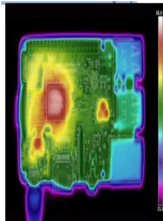
Figure 4: Raspberry Pi 3B+ thermal image (above)
