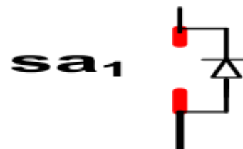
Fig.5. Shows the fault occurred due to the IGBT in open condition.
