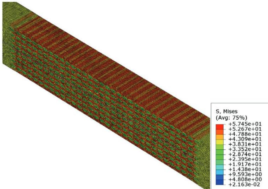
Figure 9: Von Mises stress concentration around discontinuities.
