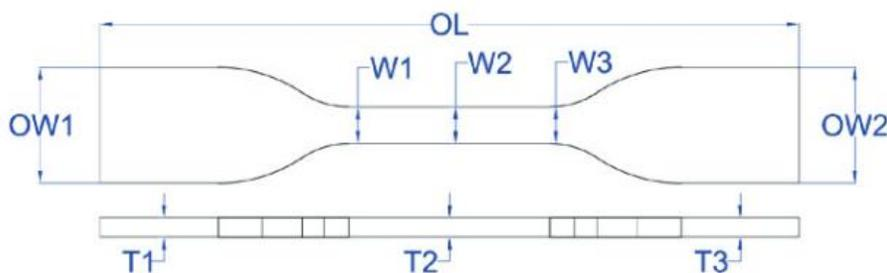
Figure 4: Measurement locations of the FDM specimens
