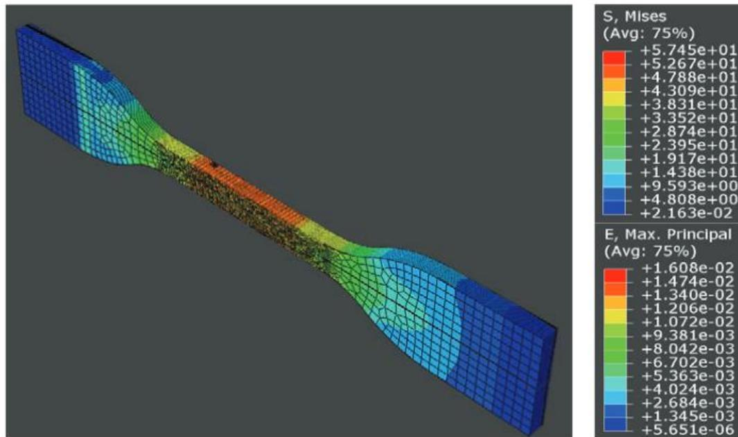
Figure 8: Von Mises stress distribution on the model with discontinuities with legends of Von Mises and principle strain.
