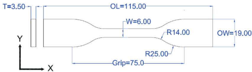
Figure 2: Created specimens' CAD model, dimensions in mm
