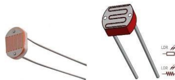
Fig. 6: LDR (Light Dependent Resistor) or Photo resistor
