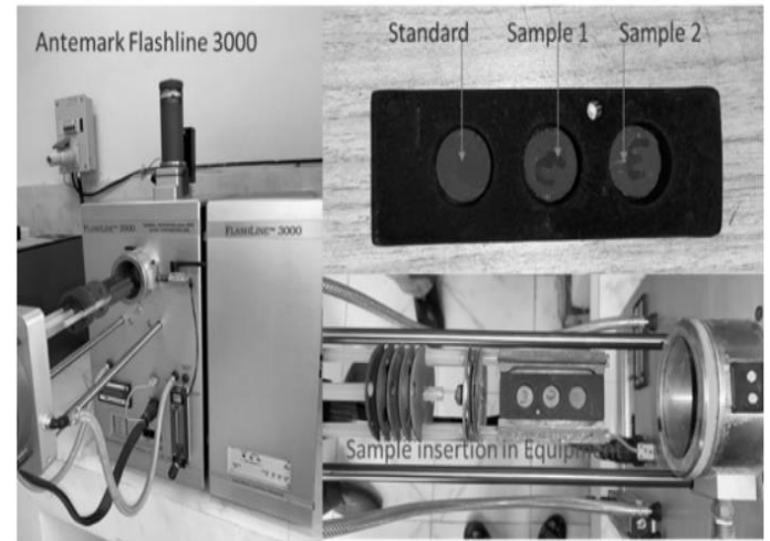
Figure 3: Set-up for Thermal Conductivity Measurement by Laser Flash Method.
