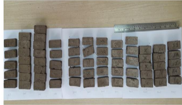
Figure 2: Waste Propellant Impregnated Fire Clay Brick.
