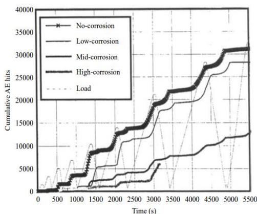
Figure 3: RC beam AE hit totals over time (in seconds) (41);
