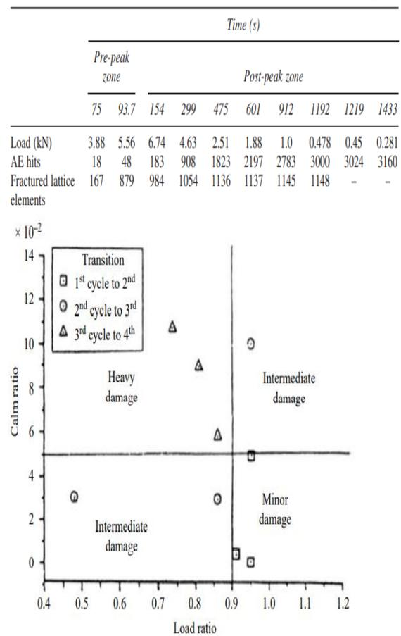
Figure 8. Classification of AE data by the load ratio and calm ratio [39,43]
