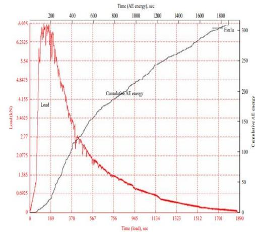
Figure 12. Variation of AE energy with time and load during concrete fracture [34].
