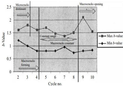
(Top) and (Bottom) channels 3 and 7 b-value variations during the course of the experiment are shown in Figure 2. The arrows on the vertical lines depict the various phases of cracking [21].
