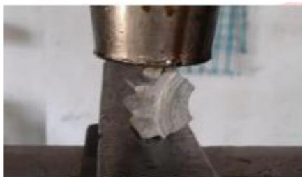
Fig.3 Testing of tangential load arrangement of gear
