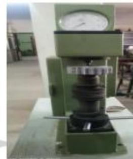
Fig.4 Brinell hardness tester
