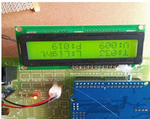
FIG 3.1.3 WHEN SOLAR PANEL IN LIGHT MODE
