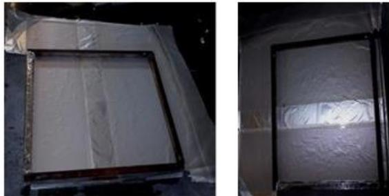
*Figure 1: Aluminum foil is wrapped around the frame.*
