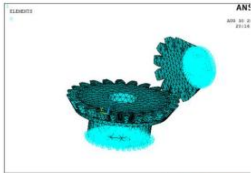
Fig: Applied fixed constraints on bevel gear
