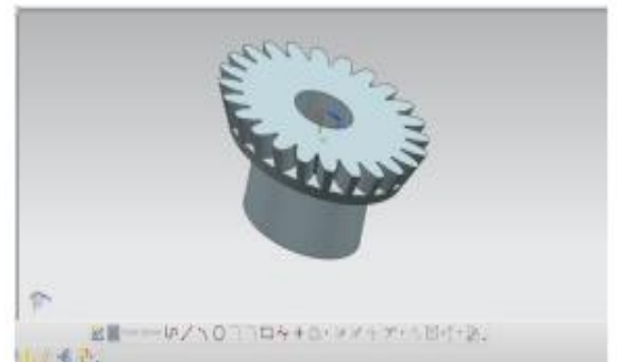
Fig: final model of the bevel gear
