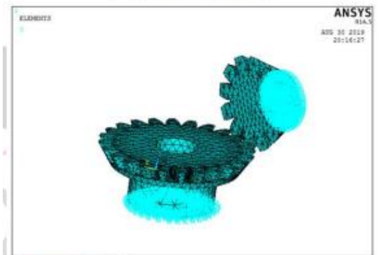
Fig: Applied fixed constraints on bevel gear
