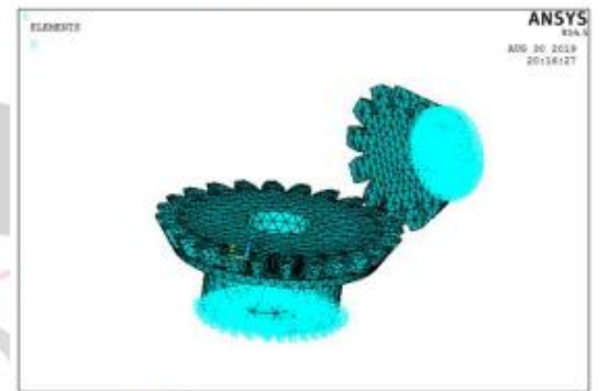
Fig: Applied fixed constraints on bevel gear
