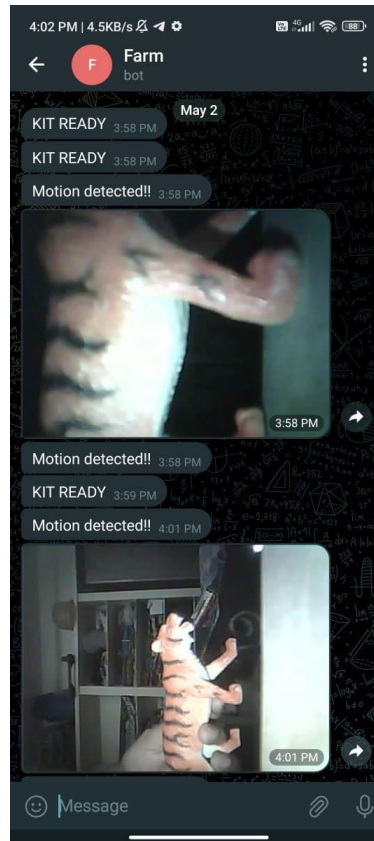
Figure 8: Message Received through Telegram to the Farmer when animal enters the Farm
