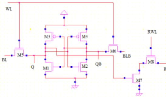
Fig.4. Conventional 8T SRAM cell
