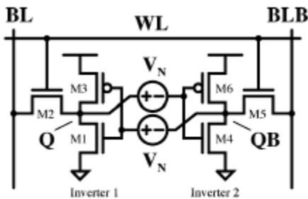
Fig.2. Standard set up for finding SNM [7]
