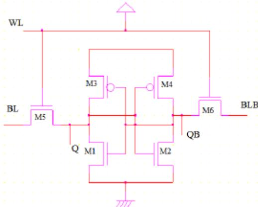
Fig.1. Conventional 6T SRAM cell
