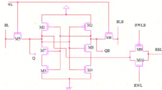
Fig.5. Proposed 10T SRAM cell
