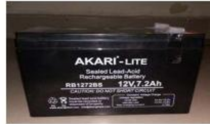
Figure 7: Battery pack for Electrical Units
