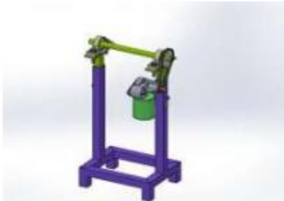
Figure 6: Frame for holding Support Rollers
