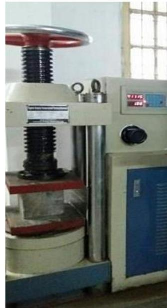
Figure 7.1 Compressive strength test
