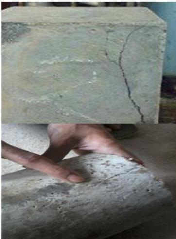
Fig . 7.2 Cracks formed in the specimen
