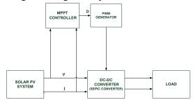
Fig. 6: Overall setup for implementing MPPT
