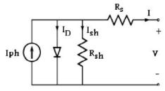
Fig.1: Equivalent Circuit of a Solar Cell The I-V characteristics of the solar cell is given by which allows for the development of robust MPPT the equation
