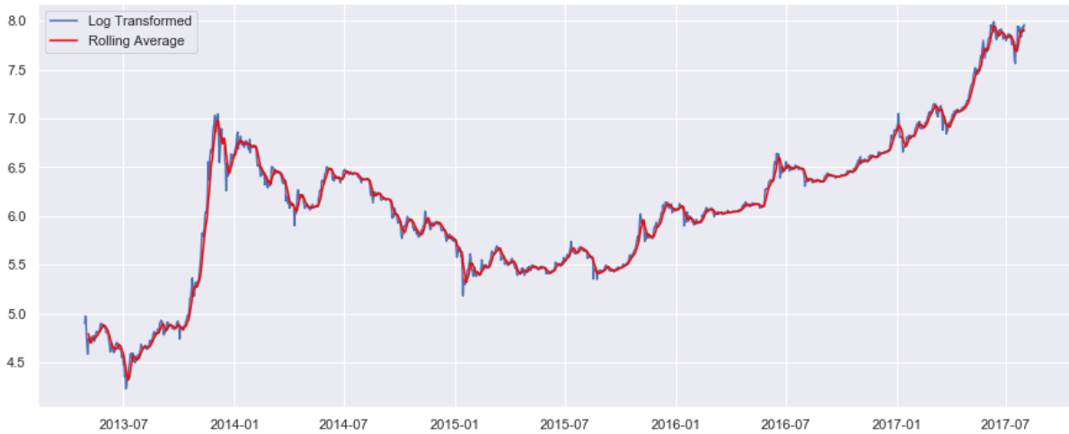
Figure 5: The plot displays a time series data (in blue) after applying a rolling average (in red) with a window size of 7, providing a smoothed representation of the original data.
