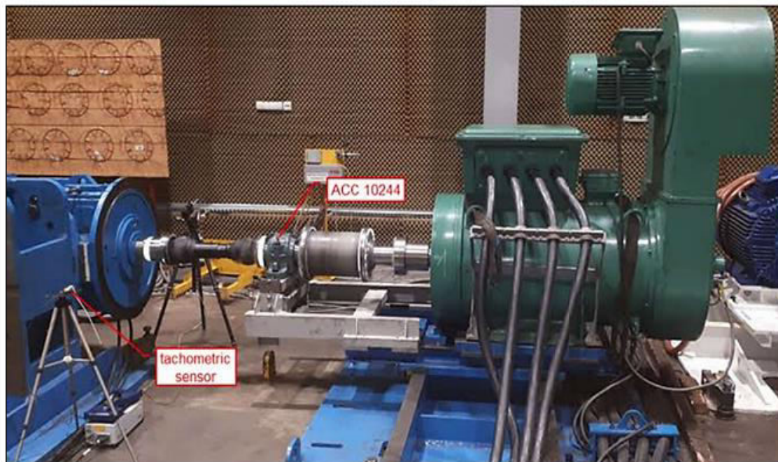
Figure 6: Location of ACC 10244 Vibrational sensor and tachometric sensors
