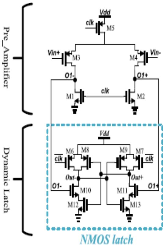
Figure 1(a): NMOS two-stage dynamic comparator.
