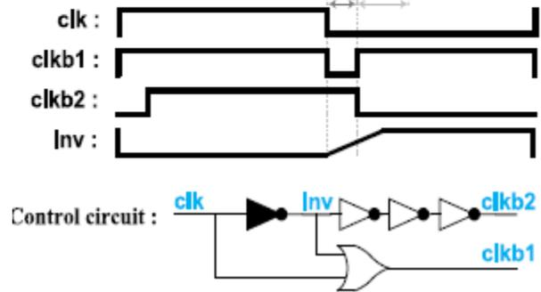
Figure 2(b): Output Waveform and Clock Signal.
