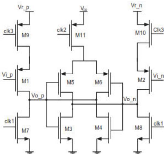
Figure 4: schematic of the Proposed Comparator
