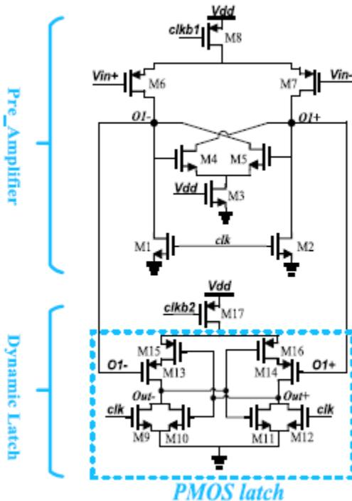
Figure 2(a): PMOS two-stage dynamic comparator.
