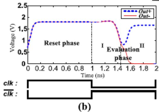
Figure 1(b): Output Waveform and Clock Signal.
