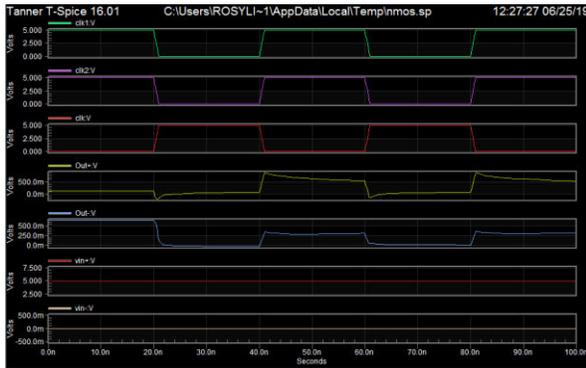
Figure 6: Typical NMOS output waveform and clock signal.
