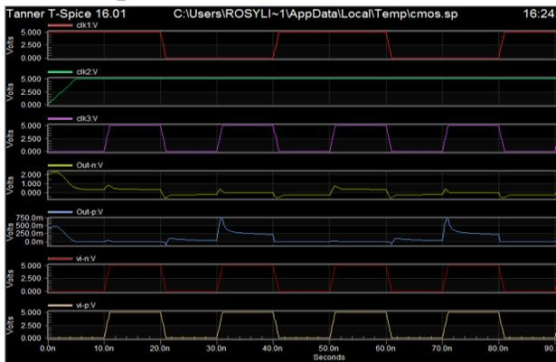
Figure 4.3: Output Waveform of Proposed CMOS Comparator.
