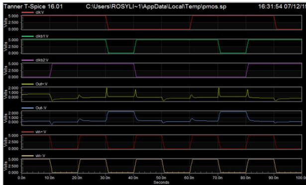
Figure 7: Typical PMOS output waveform and clock signal.
