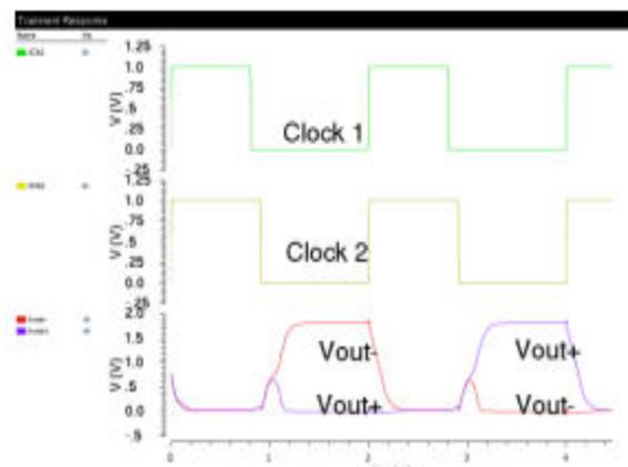
Figure 5: Output waveform showing the swing of the proposed comparator
