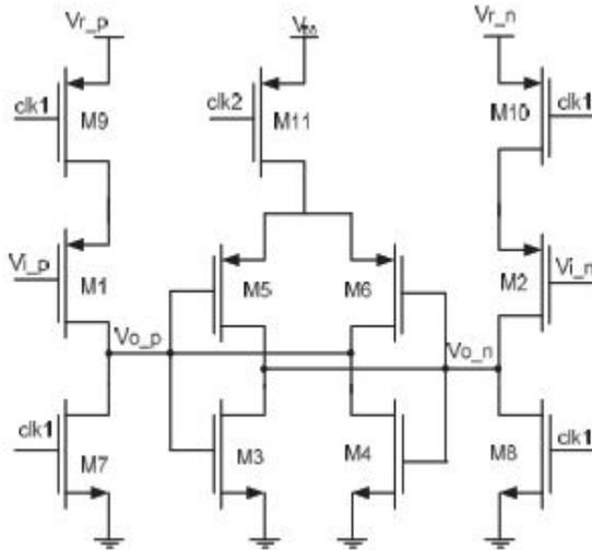
Figure 3: Differential dynamic comparator
