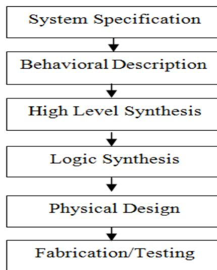
Fig.1.1: VLSI Design Flow
