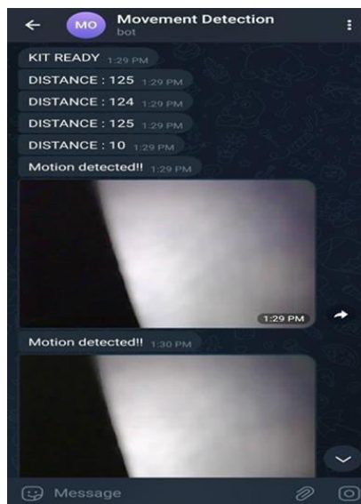
Figure 4: Shows the captured images of movement detection where every time the PIR sensor detects motion, as seen in and the user is notified.
