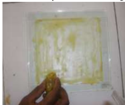
Fig: 2.3 applying Wax to the mould
