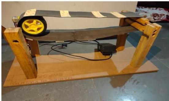
Fig 4:-Fabricated mini belt conveyor
