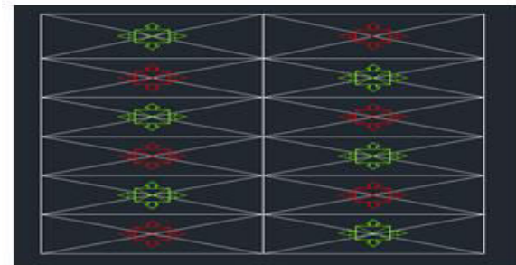
Figure: 4 Diffuser location
