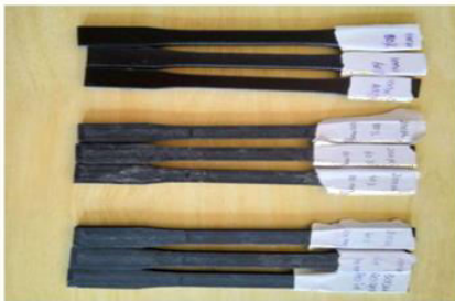
Figure 7 : Tensile Specimen (Carbon fiber PLA) (ASTM D638)
