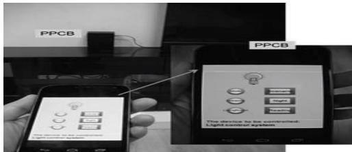
Fig.3.9 Pointing to the PPCB of the lighting control system and pressing the “Mode” button (at this point, the state of the lighting control system is powered on in scenario control mode with no single lighting control available).
