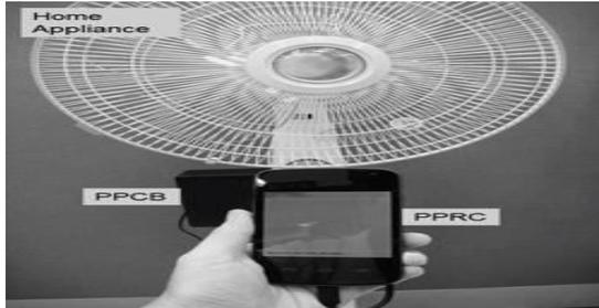
Fig.3.6 Pointing to the PPCB of the fan (at this point, the state of the fan is powered off).
