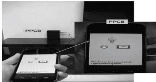
Fig.3.8 Pointing to the PPCB of the lighting control system (at this point, the states of all lights are powered off).
