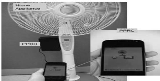
Fig.3.7 Pointing to the PPCB of the fan and pressing the “Power” button (the state of the fan is powered on in normal mode and a moderate wind speed).
