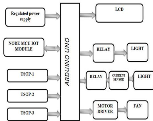
Fig. 3.3 : Block diagram of Control box
