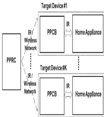
Fig 3.1 System architecture of the proposed system
