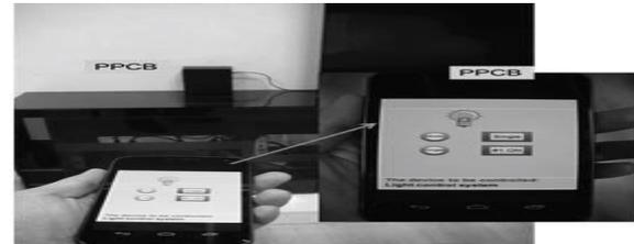
Fig.3.10 Pointing to the PPCB of the lighting control system and pressing the “Mode” button again.
