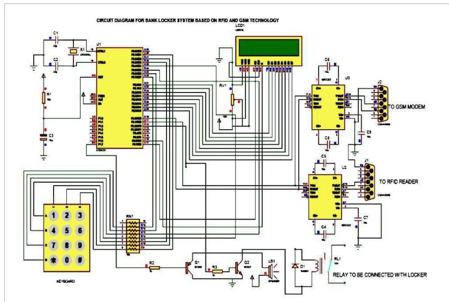
Fig-2: Circuit diagram of Bank locker system
