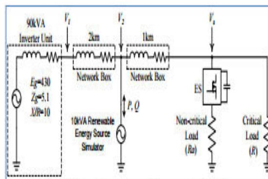
Fig. 9: Schematic overview of the experimental set up
