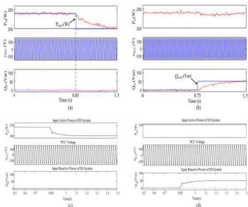
Fig. 9. Experimental and simulation results of the ES-2 system. (a) Experimental results of  $P_{inj}$  changing from 240 to 200 W whilst  $Q_{inj}$  is set to 0. (b) Experimental results of  $Q_{inj}$  changing from 0 to 50 Var whilst  $P_{inj}$  is set to 240 W. (c) Simulation results of  $P_{inj}$  changing from 240 to 200 W whilst  $Q_{inj}$  is set to 0. (d) Simulation results of  $Q_{inj}$  changing from 0 to 50 Var whilst  $P_{inj}$  is set to 240 W.
