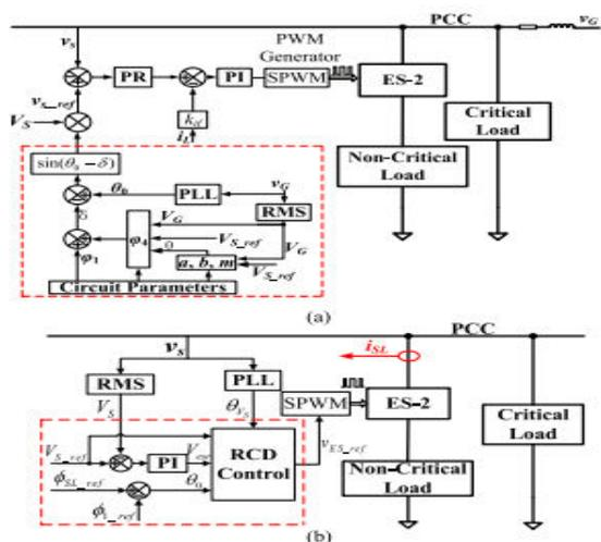
Fig. 2. ES-2 control diagrams for (a)  $\delta$  control and (b) RCD control.
