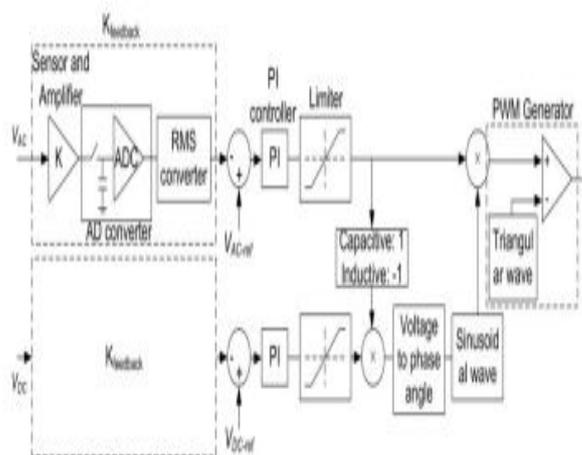
Fig. 4: Block diagram for electric spring control
