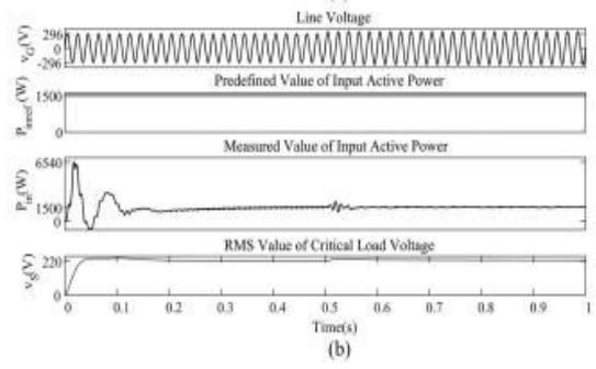
Fig. 6. Transient ES-2 responses to a change of the line voltage with  $P_{inref} = 1.5$  kW. (a) From 240 to 210 V. (b) From 210 to 240 V.
