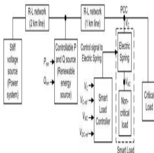
Fig. 5: Block diagram of the test system with Electric Spring
