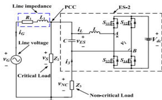
Fig. 1. Topology of ES-2 and associated circuitry.
