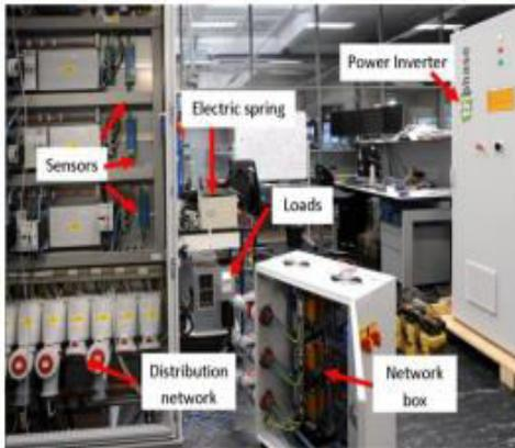
Fig. 10: Photograph of the experimental set up with major components shown
