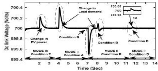
Fig. 6. Variation of dc link voltage scenario I
