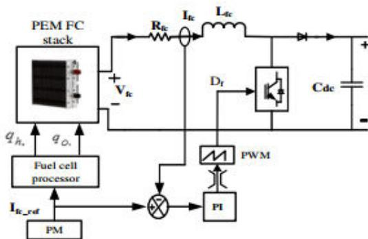
Fig. 3. PEM fuel cell with boost converter
