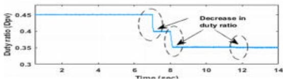
Fig.9. Variation of PV boost converter duty ratio scenario I
