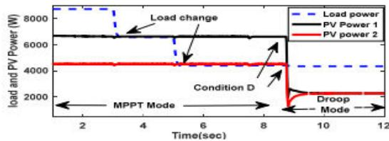
Fig. 18. PV1, PV2 and load powers.
