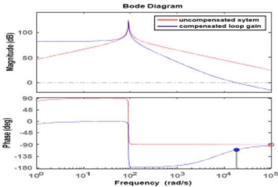
Fig.4. Bode plot of compensated loop gain and uncompensated loop gain
