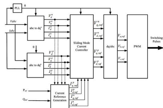
Fig.5 Block diagram of current control strategy where the state variable is X, the control input U and grid voltage  $V_g$
