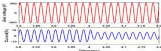
Fig. 12. Load voltage (L-L) and load current scenario I
