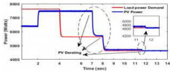
Fig.7. Variation of PV power and load power
