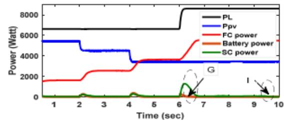
Fig. 14. PV, SC, FC, battery and load power scenario II
