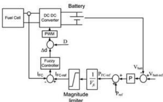
Fig. 5 Control of fuel cell subsystem.
