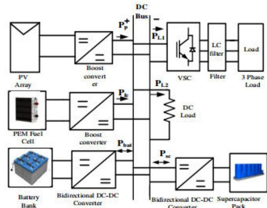
Fig. 1. Hybrid AC/DC Microgrid configuration 1
