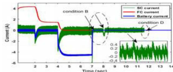
Fig.10. Variation of SC, FC and battery currents scenario I
