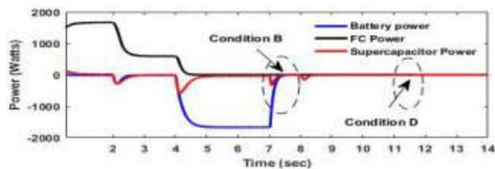
Fig.8. Variation of Battery, SC and FC powers scenario I
