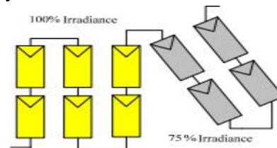
Fig. 7 Homogeneous Shading (different tilt angle)
