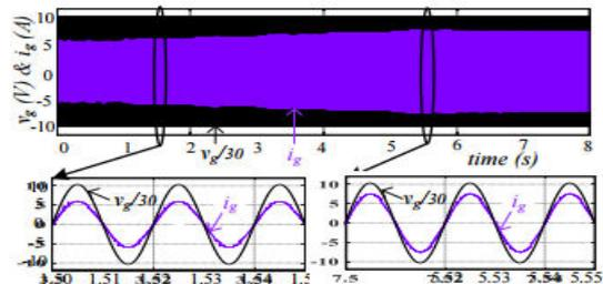
Fig. 7. Simulated waveform:  $v_g$  and  $i_g$  and their magnified views
