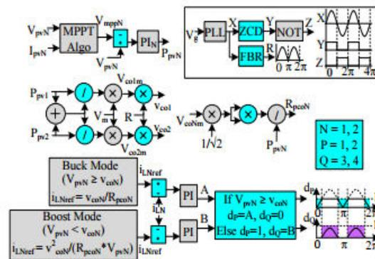
Fig. 5. Control configuration of the proposed inverter
