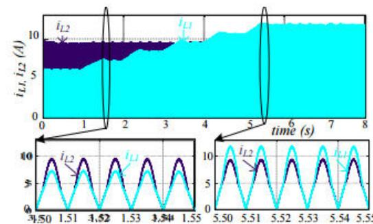
Fig. 8. Simulated waveform:  $i_{L1}$  and  $i_{L2}$  and their magnified views
