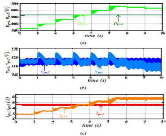
Fig. 6. Simulated waveform: Variation in (a)  $P_{pv1}$  and  $P_{pv2}$ , (b)  $V_{pv1}$  and  $V_{pv2}$ , (c)  $I_{pv1}$  and  $I_{pv2}$  during entire range of operation
