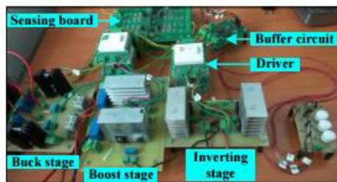
Fig. 10. Experimental prototype of the proposed inverter
