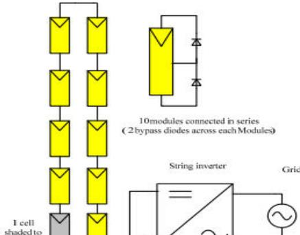
Fig. 9 Series connection of 10 modules
