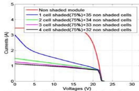
Fig.5 Effect of different number of cells shading
