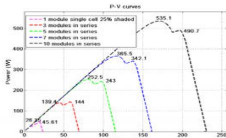
Fig. 10 Effect of partial shading in series connection
