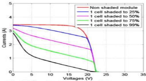
Fig. 4 Effect of partial shading in I-V curves
