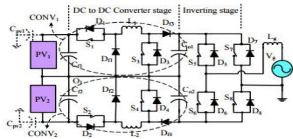
Fig. 1. Dual Buck & Boost based Inverter (DBBI)
