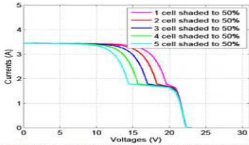
Fig 6. Effect of using bypass diodes across each solar cell
