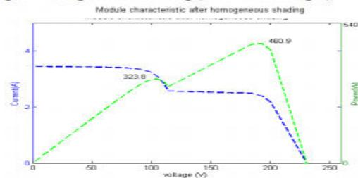
Fig 8: Effect of Homogeneous shading in string (fig.7) characteristics.
